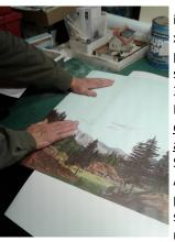
The most popular size is the 3/16" thick, 24" x 48". Gather your GF, photo, and some spray adhesive. (I like 3M 77Spray adhesive). It's recommended to do this outdoors or in a well-ventilated area! Spray your Gatorfoam AND the back of the photo with the adhesive and let sit for the recommended time.
